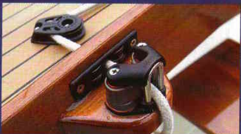
Decent ball race blocks and modern cam jammers make life easier elsewhere
