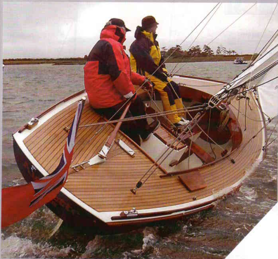
Decent ball race blocks and modern cam jammers make life easier elsewhere
